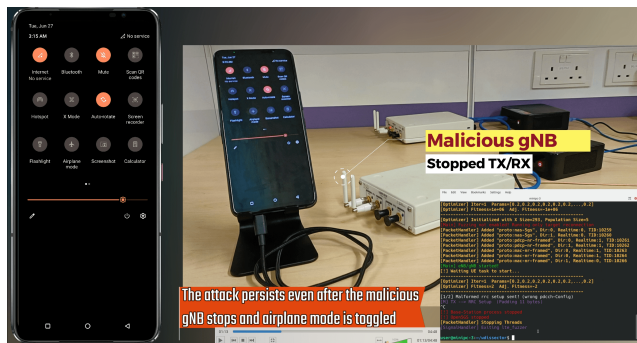
Video 1: Demonstration of "Disabling 5G connection via Invalid RRC pdccch-Config" (CVE-2023-33042). Youtube Video URL: https://youtu.be/DiGqwgBCSXM
