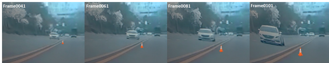
Fig. 23. A sequence of zoom-in image frames depicting the change in size and position of the cone over time. The shown frames are 20 frames (two-thirds of a second) apart.
