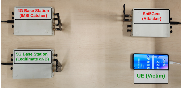
Figure 3: Physical setup showcasing a rogue 4G base station (IMSI catcher), a legitimate 5G base station, the SNI5GECT attacker device, and the victim UE (OnePlus Nord CE 2).
